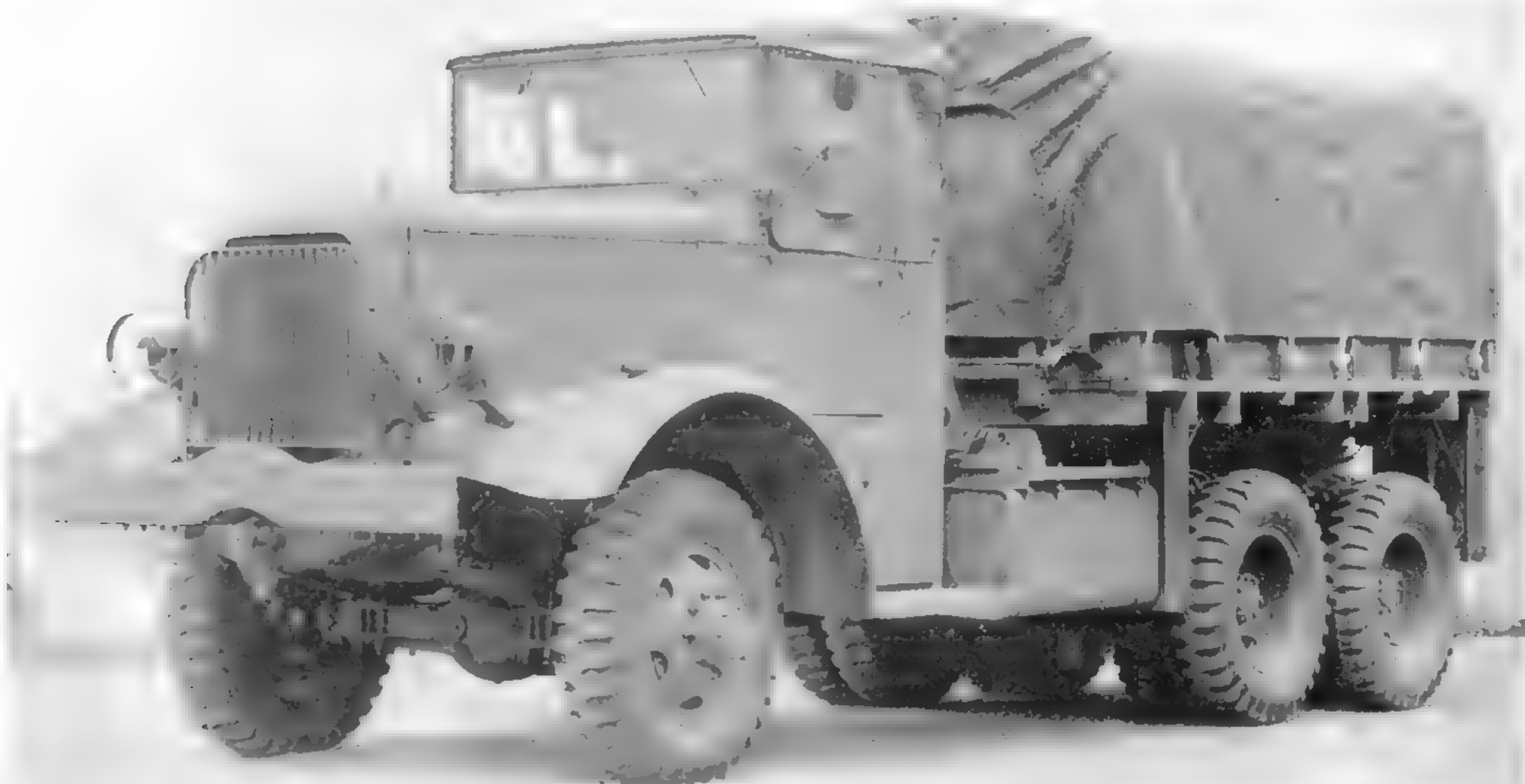
The front pintle hook can be seen clearly in this photograph, as can be the liquid container racks above the fuel tank. This imposing vehicle is the Mack NM-6. (Photo courtesy of the Mack Trucks Historical Museum)
